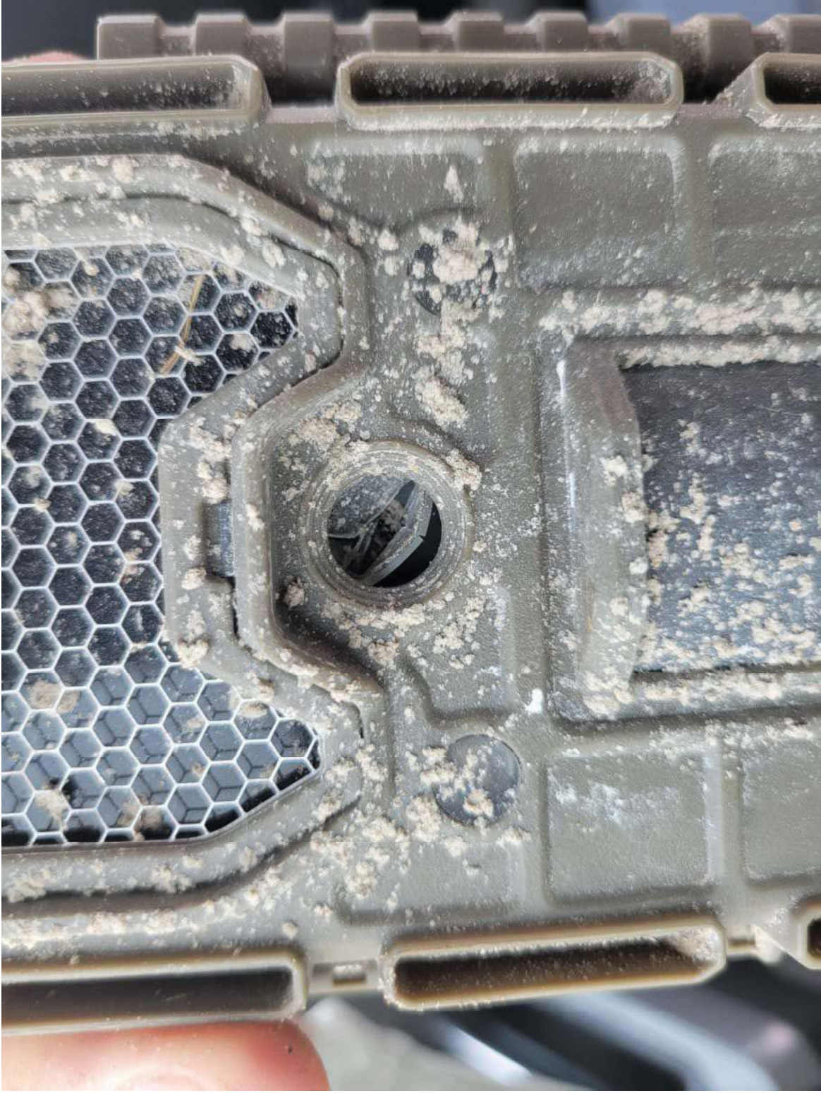
Figure 15. Game camera from WIPL 1 showing completely cracked camera lens after pebble was removed post-launch on June 6, 2024.
